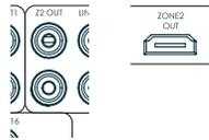
The Z2 out HDMI connector can be used to connect the output of the Receiver to a system located in a second room.
