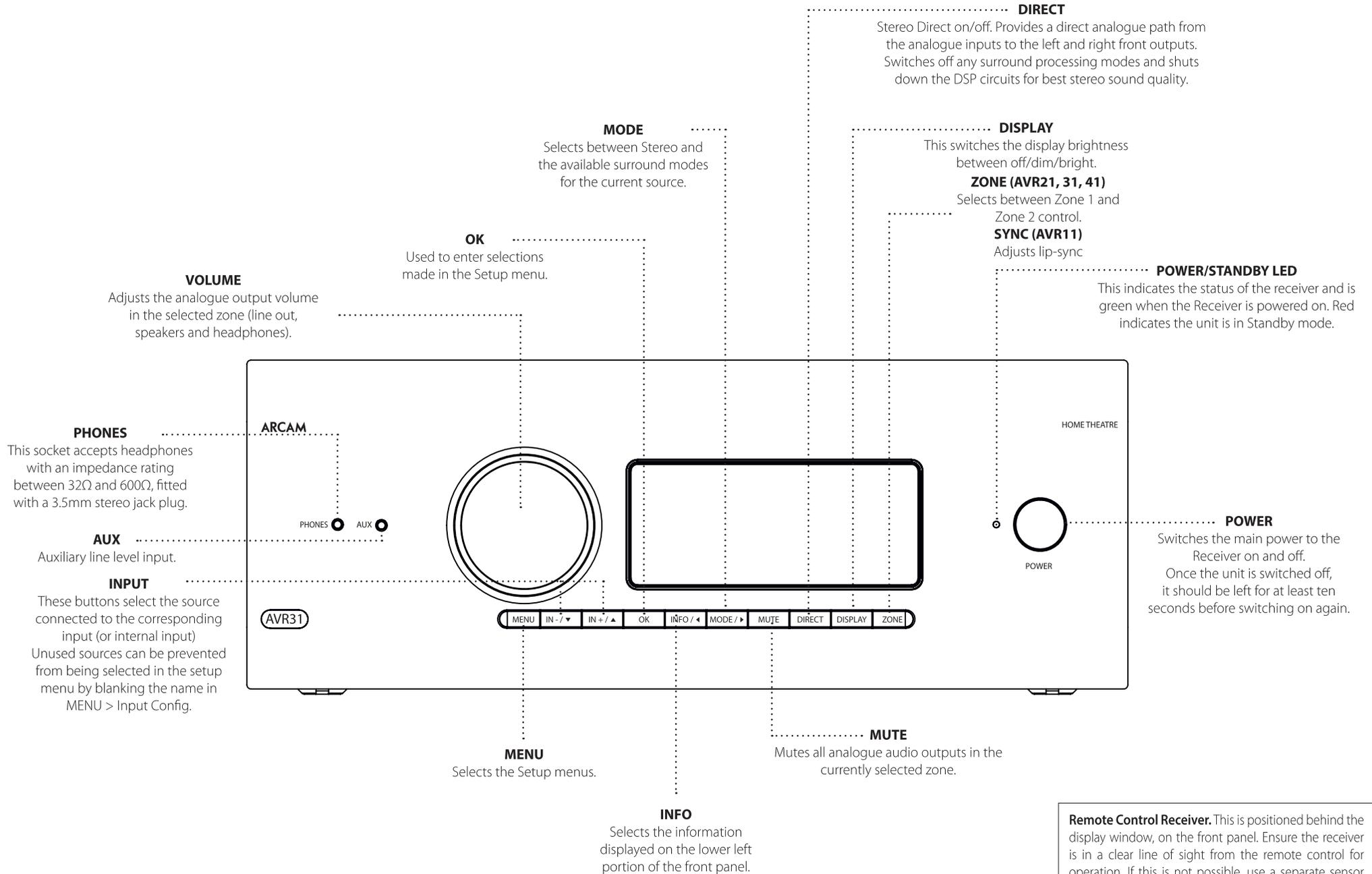
**Remote Control Receiver.** This is positioned behind the display window, on the front panel. Ensure the receiver is in a clear line of sight from the remote control for operation. If this is not possible, use a separate sensor connected to the **Z1 IR** input on the rear panel.
