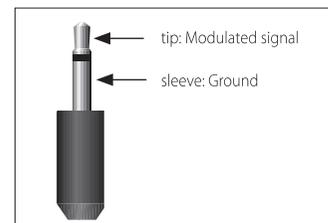
The infrared inputs (**Z1 IR** and **Z2 IR**) allow the connection of external IR receivers, either when the Receiver front panel IR receiver is fully or partially obstructed or to allow the use of a remote control in Zone 2.
