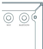
If using the Wi-Fi or Bluetooth features of the Receiver, please attach the single antenna for the Bluetooth and the two antennas for the Wi-Fi.
