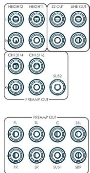
All preamplifier analogue outputs are buffered, have a low output impedance, are at line level and follow the Zone 1 volume control setting. They are able to drive long cables or several inputs in parallel if required.
