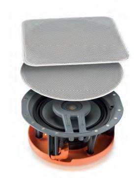
Trimless grilles are held in place magnetically by high power Neodymium magnets. A choice of interchangeable round or square grilles is offered by the in-ceiling/wall models, and for the perfect blend with any environment, all grilles are paintable: additional scrim material is provided.
